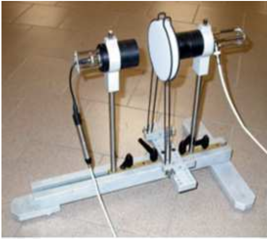
Fig. 3. Test rig for Tortuosity measurement (ENDIF, Italy) and Effect of tortuosity on Sound Absorption
