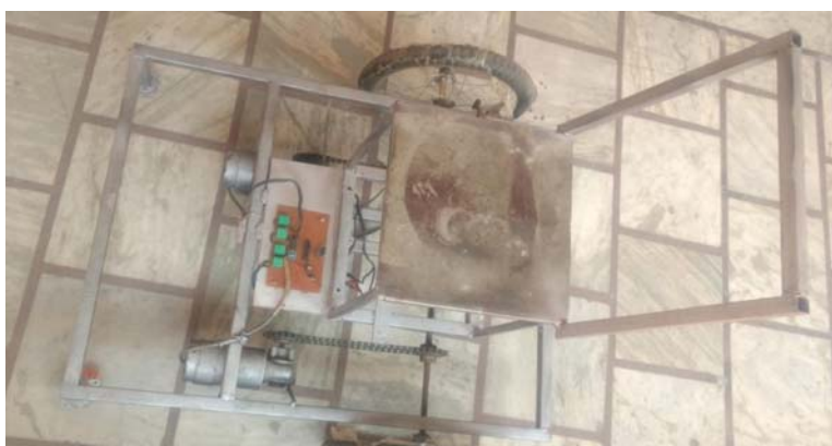
Fig. 4 Traditional voice control wheelchair
