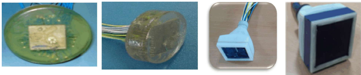
Fig. 5: (a) 5×5 sensor array (1.8 × 1.8 cm); (b) 6×6 sensor array (1.8 × 1.8 cm); (c) 128 Element 2D array (6.2 × 6.2 cm); (d) 169 element 2D array (6.2 × 6.2 cm)
