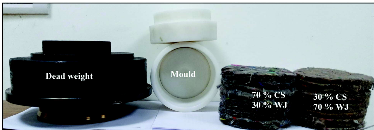
Fig. 1. Prepared samples with mould and dead weights used to apply pressure
