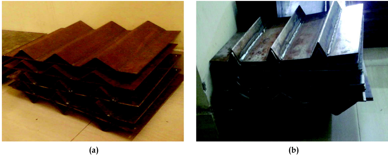
Fig. 1. Fabricated plates for measuring insertion loss: (a) Set A corrugated plates, (b) Set B corrugated plates
