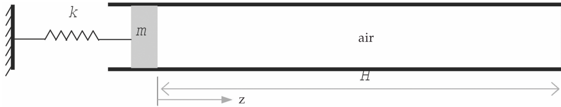
Fig. 8. A simple model to illustrate coupling of one membrane mode with axisymmetric cavity modes.
