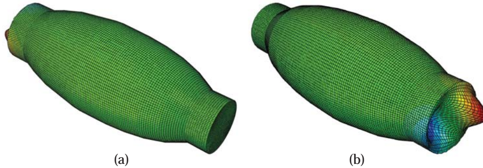
Fig. 10. A non-axisymmetric Thoppi mode showing weak vibro-acoustic coupling; (a). view from Karanai side and (b). from Thoppi side.
