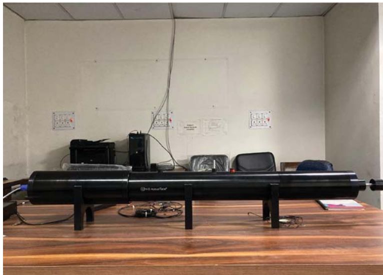
Fig. 3. Impedance tube system at National Physical Lab, New Delhi.
