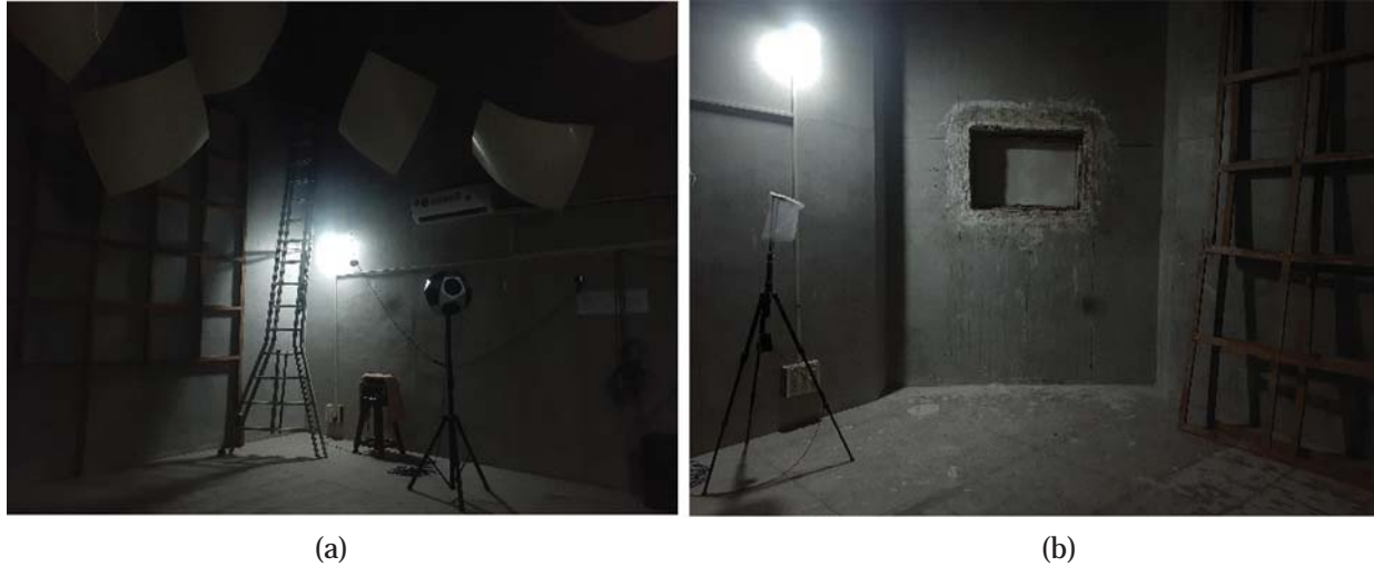
Fig. 2. (a) Reverberation chamber without sample and (b) Reverberation chamber with Sample installed at National Physical Lab, Delhi
