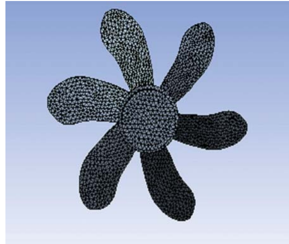
Fig. 3. Meshed model of optimized propeller
