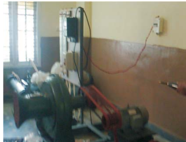
Fig. 2 Experimental Setup for aeroacoustic Measurements
