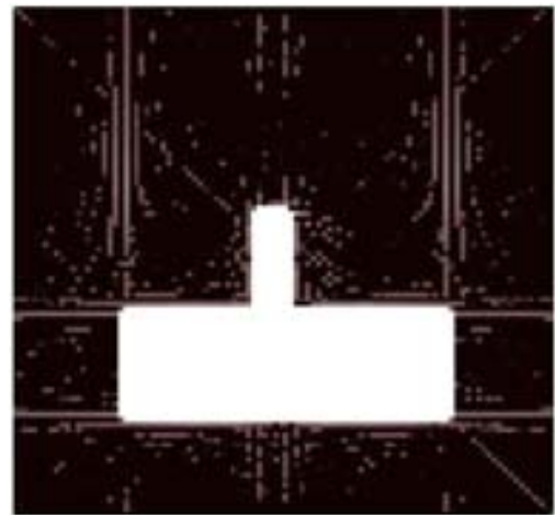
Fig. 7c. Shapereconstructed, by applying Inverse Radon function on Fig. 7b
