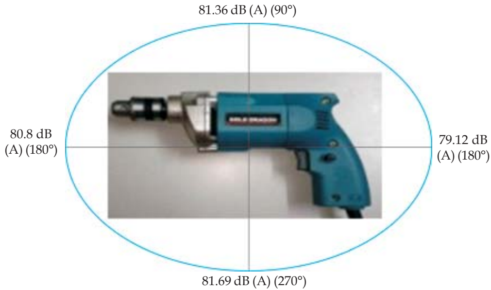
Fig. 2. Directivity of a hand drill
