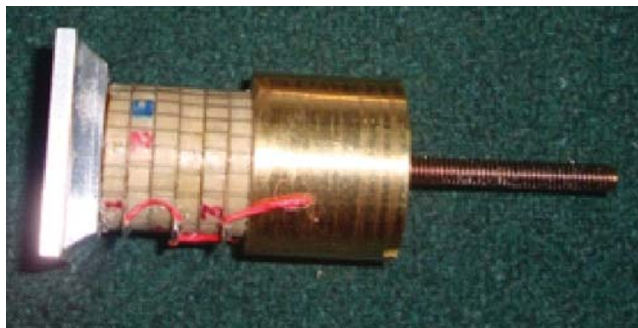
Fig. 6. A designed and developed prototype 1-3 piezocompositetonpilztransducer.
