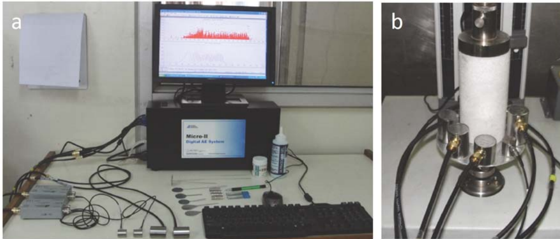
Fig. 1. Experimental setup for AE measurements: (a) Acoustic emission monitoring system; (b) Snow sample under testing.
