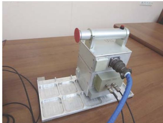
Fig. 2. Measuring block with changeable water container
