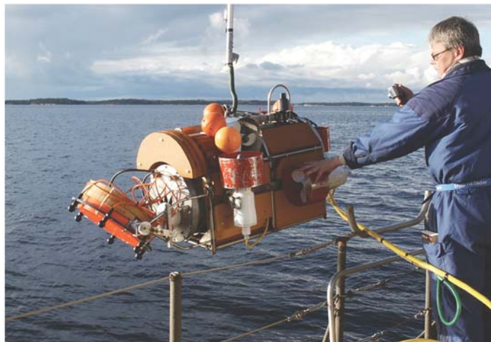
Fig. 1. Experimental set up using the ROV of FOI, PLUMS (Platform for Underwater Measurement Systems) where TOPAS 120 parametric sonar was installed. ROV navigation was monitored by a long baseline.
