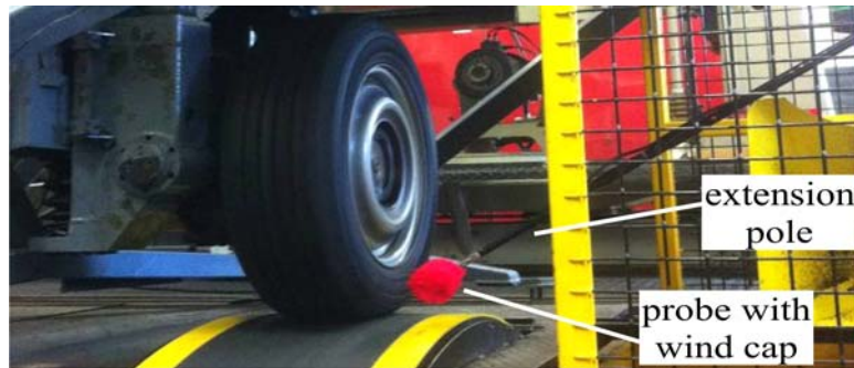
Fig. 7. Tyre on the roller bench. The surface is scanned using an extension pole.
