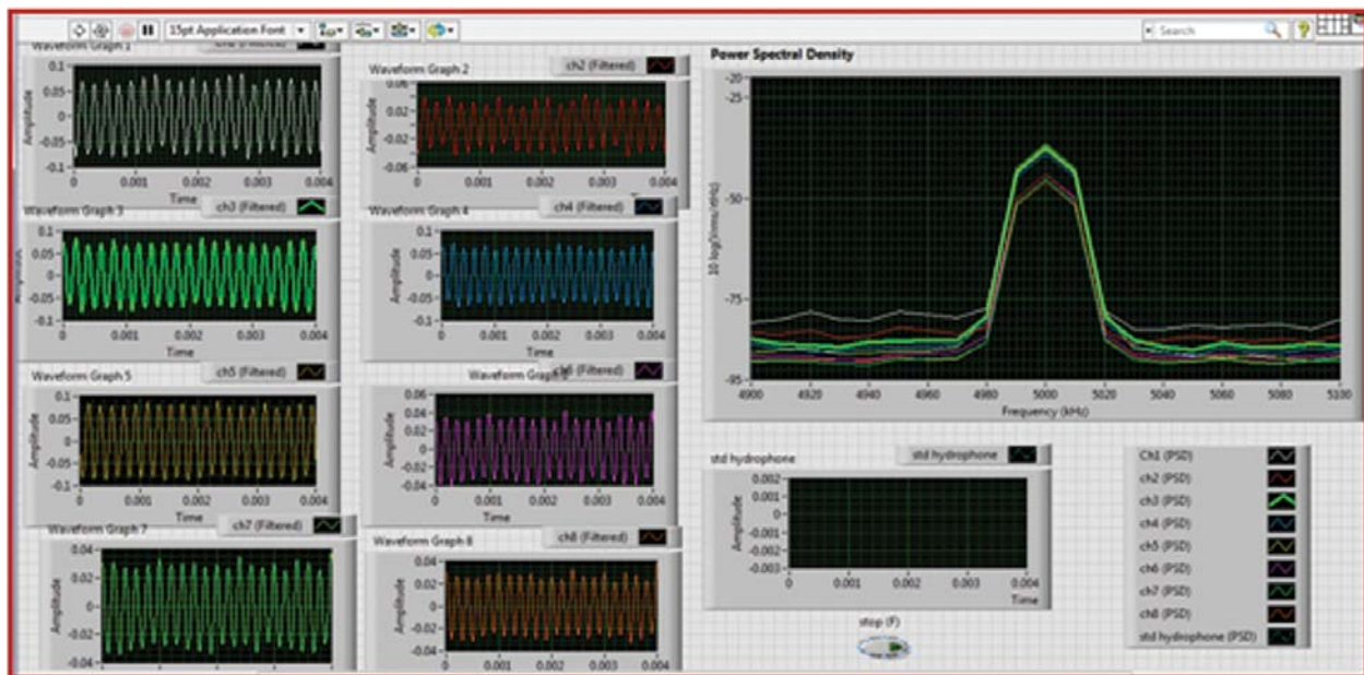
Fig. 8. Observed time signal from the array when insonified at 5000Hz
