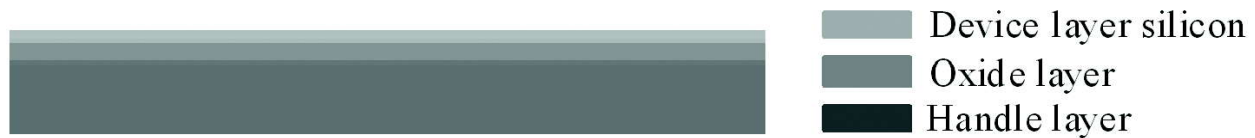
Fig. 3. Figure showing schematic representation of SOI (Silicon-On-Insulator) wafer and its nomenclature.
