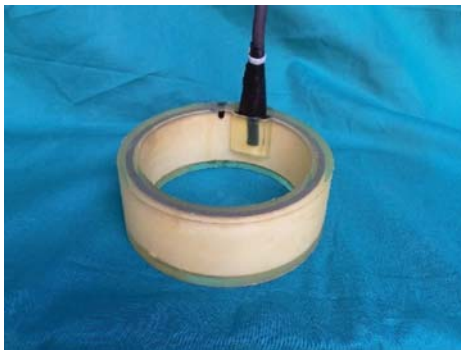
Fig. 5. PU moulded transducer.
