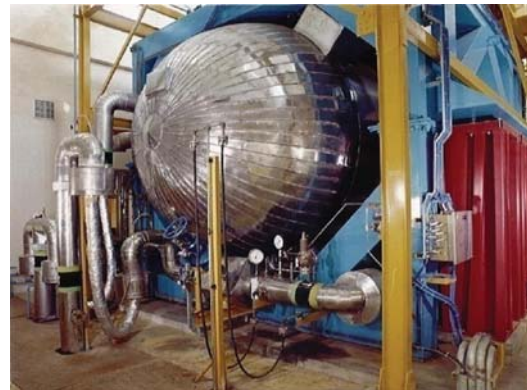
Fig. 8. Pressurised acoustic test chamber [9].
