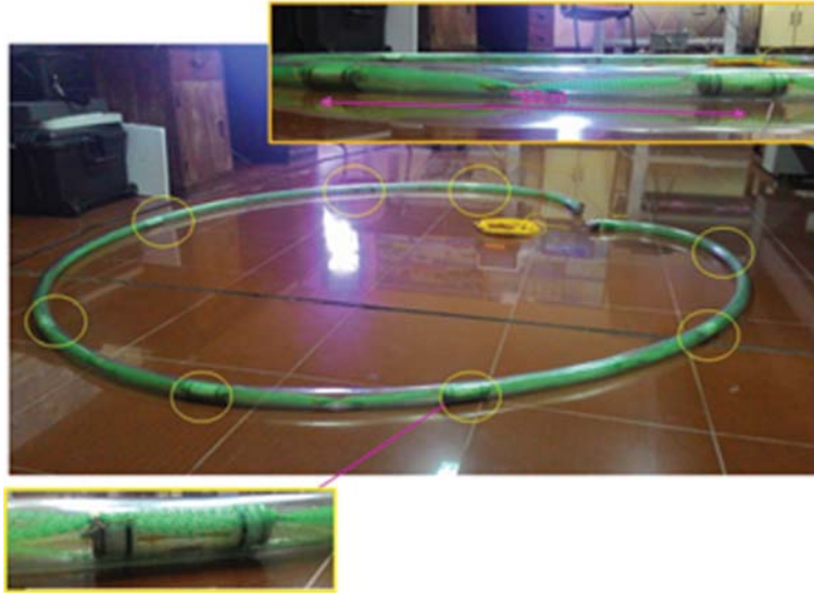
Fig. 4. Eight element array in 32 mm PU tube, sensor positions circled and enlarged
