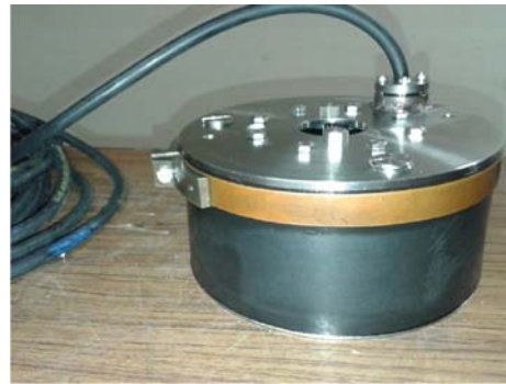
Fig. 6. Transducer with oil filled rubber boot.
