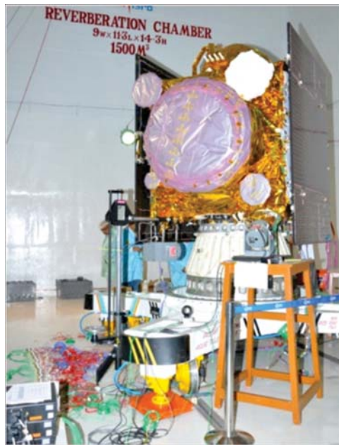
Fig. 8. spacecraft modal test setup in RC
