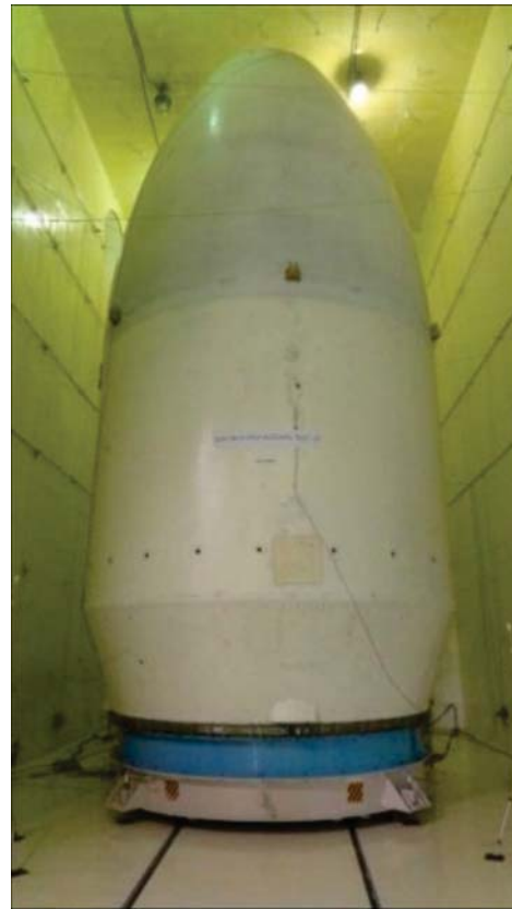
Fig. 1b. Composite Payload Fairing with Ogive nose cone in Reverberation chamber
