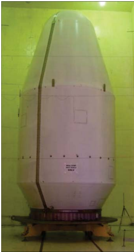
Fig. 1a. Composite Payload Fairing with straight nose cone in Reverberation chamber
