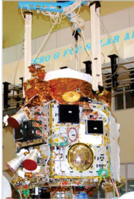
Fig. 6. Micro vibration measurement test setup
