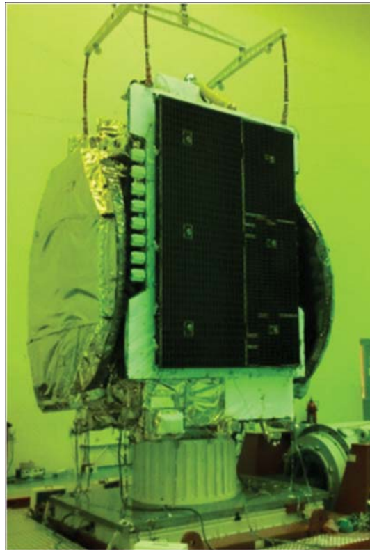
Fig. 1. Lateral axis sine vibration test setup
