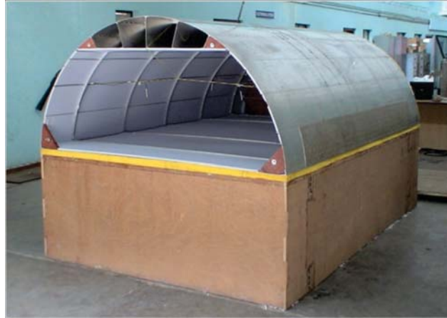
Fig. 9. Melamine foam installed segmented fuselage
