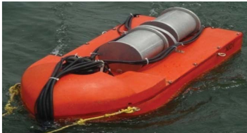
Fig. 2. Tow fish integrated with Transmitter and hydrophones
