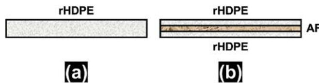
Fig. 2. (a) Type 1-Neat rHDPE (b) Type 2-rHDPE/AF/rHDPE sandwiched composite.
