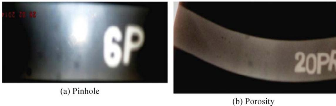
**Fig. 8.** Radiographic film shows (a) pinhole and (b) porosity defects.
