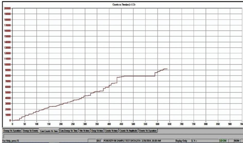
Fig. 6. Emission continuing during load hold indicates instability.
